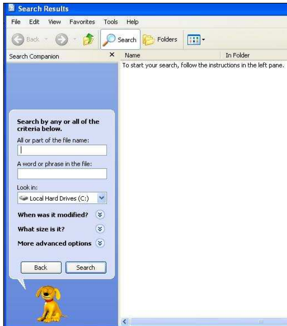
Figure 21: A snapshot of the Windows 'Search' tool. A weakness found with this searching method, is the elapse time from the time the search is employed to the time all search results are returned. Sometimes users wait for their results only to find that the search criteria entered is too narrow, returning no results, or too broad, returning too many results.
