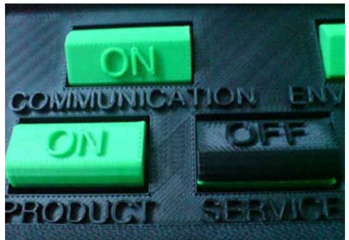
■ To mimic on/off switches or buttons, multi-colored rollers were constructed.
