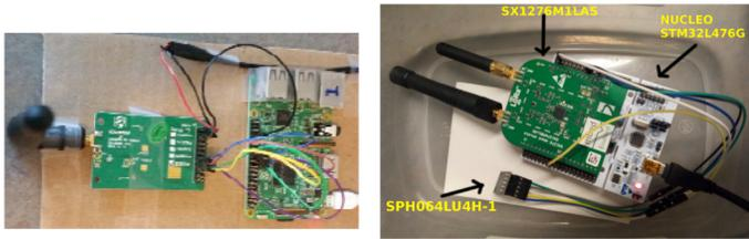
(a) Raspberry Pi LoRa gateway. (b) IoT device with LoRa shield.
