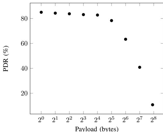
Fig. 6: Effect of payload size on PDR.
