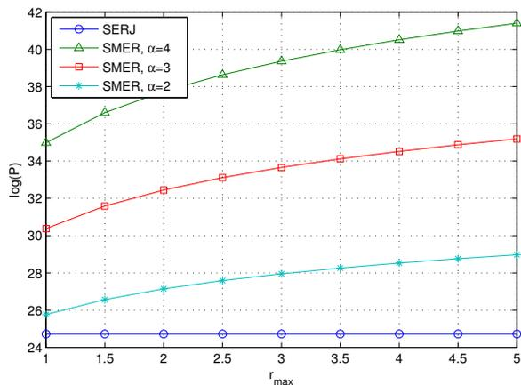
Fig. 5: Power consumption of SERJ and SMER versus  $r_{max}$  for various values of  $\alpha$  and when  $n_E = 5$  eavesdroppers are present. The performance of SMER is closely dependent on the uncertainty in the locations of the eavesdroppers, while the performance of SERJ does not depend on the locations of the eavesdroppers.
