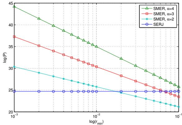
Fig. 4: Power consumption of SERJ and SMER versus the radius  $r_{min}$  of the guard region for various values of  $\alpha$  and when only one eavesdropper is present. As we allow the eavesdropper to become closer to the transmitter (i.e. as  $r_{min}$  gets smaller), the power needed to make the link secure using SMER becomes higher. On the other hand, with SERJ there is no need to assume a guard region around the transmitter.
