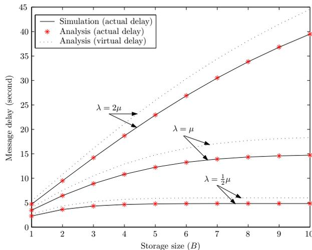
Fig. 8. Message delay for  $\gamma = 10^{-1}\mu$ .
