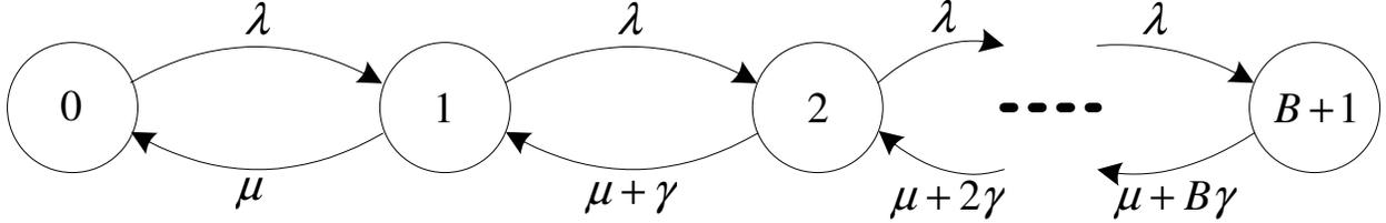
Fig. 5. A Markov chain representation of the MMS-RS.
