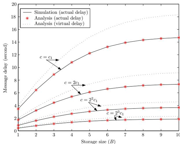
Fig. 10. Message delay for  $\lambda = \mu$  and  $\gamma = 10^{-1}\mu$ .
