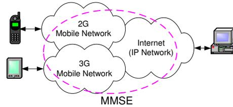
Fig. 1. General MMS architecture integrating different networks.
