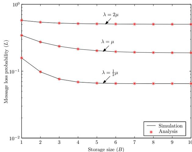
Fig. 9. Message loss probability for  $\gamma = 10^{-1}\mu$ .
