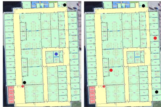
Fig. 2: *Scenario 2: A 60m by 40m floor containing several rooms and walls. The blue circle indicates the beamforming AP in Mode-1 (left), and red circles indicate omnidirectional APs in Mode-2 (right). The black circles are WiFi clients.*
