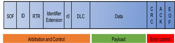
Fig. 2: Standard CAN frame structure.
