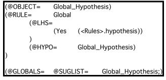
Figure 10 The top level control rule
