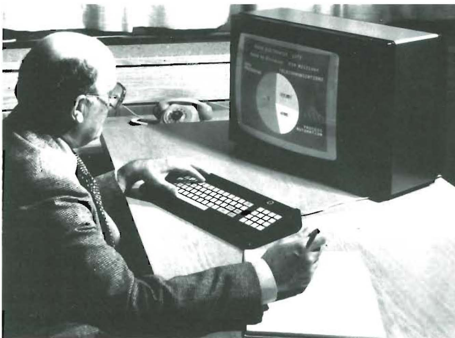
Multi-standard videotex terminal from Nokia in Finland that can decode both alpha-mosaic and alpha-geometric formats.
