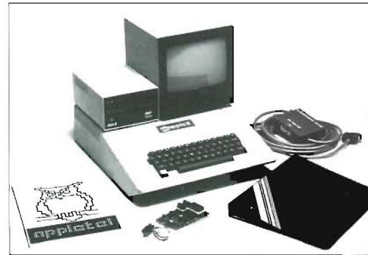
The Owl Prestel Adaptor for the Apple II Computer provides not only the facilities of a normal terminal but also the capability to record pages on disc locally and process the information in them for other purposes. Norpak in Canada are developing a similar facility to enable the Apple II to be used as a Telidon terminal.
