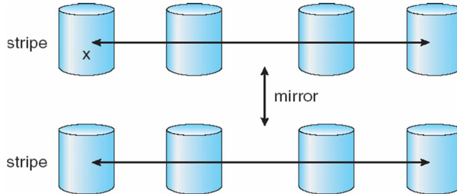
a) RAID 0 + 1 with a single disk failure.
