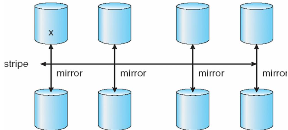
b) RAID 1 + 0 with a single disk failure.
