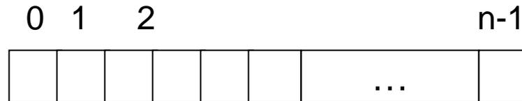
$$\text{bit}[i] = \begin{cases} 0 \Rightarrow \text{block}[i] \text{ free} \\ 1 \Rightarrow \text{block}[i] \text{ occupied} \end{cases}$$
