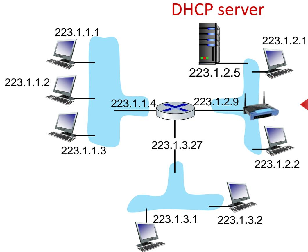
Typically, DHCP server will be co-located in router, serving all subnets to which router is attached
