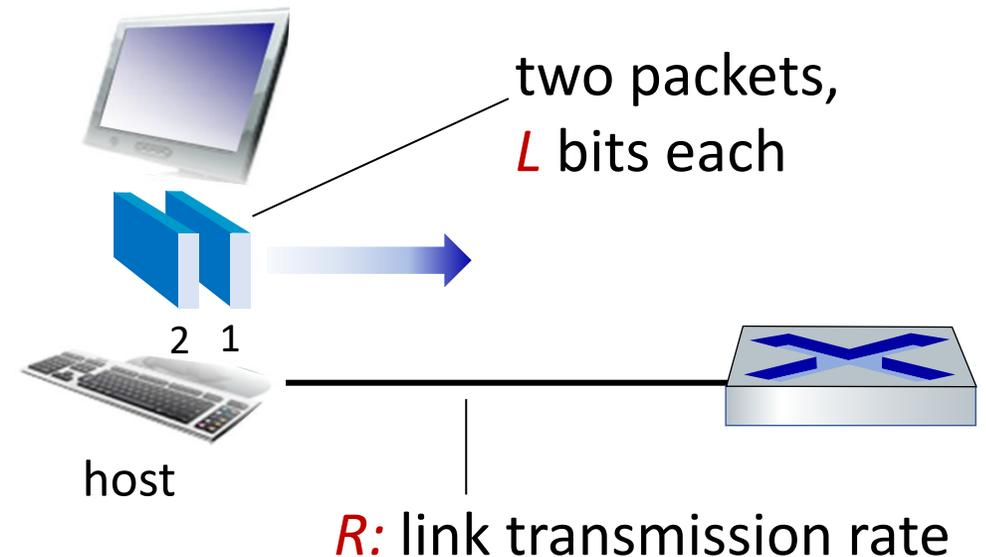
$$\text{packet transmission delay} = \text{time needed to transmit } L\text{-bit packet into link} = \frac{L \text{ (bits)}}{R \text{ (bits/sec)}}$$
