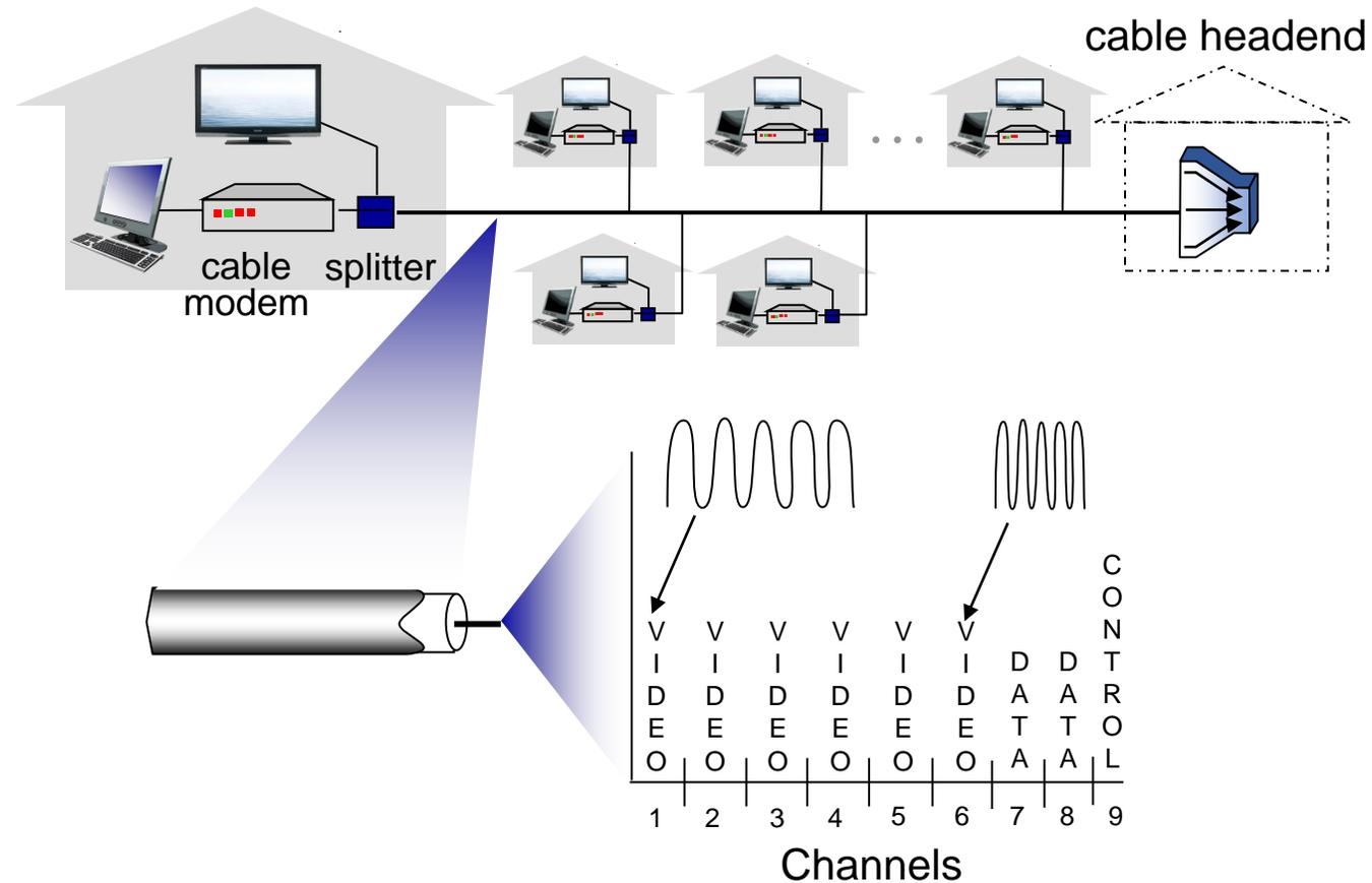
*frequency division multiplexing (FDM)*: different channels transmitted in different frequency bands
