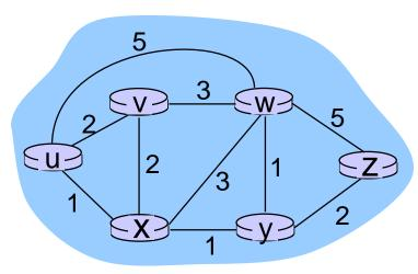
clearly,  $d_{v}(z) = 5$ ,  $d_{x}(z) = 3$ ,  $d_{w}(z) = 3$ B-F equation says:  $d_{ii}(z) = \min \{ c(u,v) + d_{ii}(z), i \}$  $c(u,x) + d_x(z),$  $C(u,w) + d_w(z)$  $= \min \{2 + 5,$ 1 + 3, 5 + 3 = 4 node achieving minimum is next hop in shortest path, used in forwarding table
