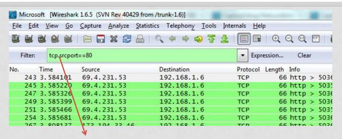
Display filter separates the packets to be displayed (In this case, only packets with source port 80 are displayed)
